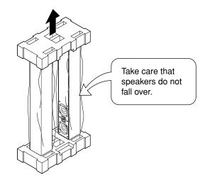
5 Lift up the speakers to remove the top protection by pressing it down, then place the speakers on the cloth.
